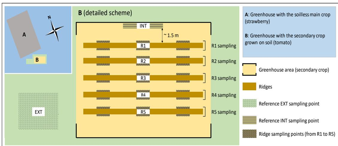
**Figure 5.** Schematic representation of the soil sampling design at the CascadeReUse System from the strawberry CRUS that reuses the drainages from the soilless main crop (strawberry) for the fertigation of a secondary crop (tomato) grown on soil (in ridges) under a plastic greenhouse.
