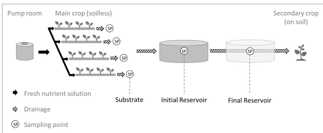
**Figure 1.** Scheme of the (a) irrigation flow, from the fresh nutrient solution until the drainage reuse on soil and scheme of the (b) CascadeReUse Systems (CRUS) from the three CRUS where drainage samples were collected. The main components of each production system and sampling points (SP) are shown in the scheme.
